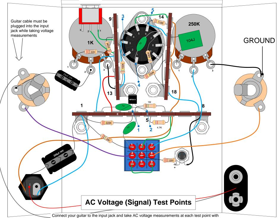
both controls turned all the way up. At each test point the AC voltage should increase dramatically each time you strum the guitar. (No strum = 0.0 VAC, Hard strum = anywhere from 10 mV to 2 V).
