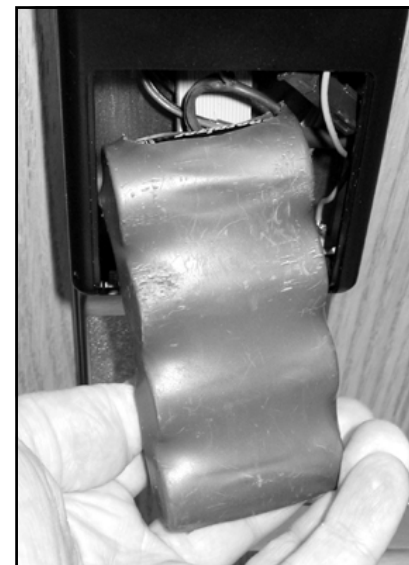
FIG. E: INSERT BATTERY PACK INTO "INSIDE HOUSING" ("SEALED" TYPE PACK SHOWN)
