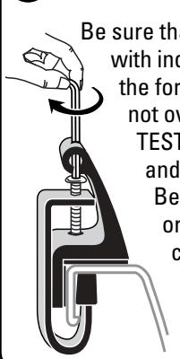
Be sure that bolt aligns with indentation in the fork block. Do not overtighten. TEST by grabbing and shaking. If BedHead slips or loses contact with rail, tighten more.
