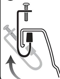
Hook rail clip under bed rail. **Position rail clip only where underside of rail is flat.** Loosen bolt more if necessary, and rotate into upright position.
