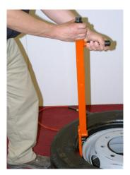
Once inserted between the bead and rim, bring tool to an upright position and ensure that you have a secure hold on the 2nd bead with the pulling foot.
