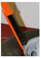
Begin tool engagement by turning the impact wrench in a counter clockwise manner. As the pushing foot begins to meet the rim ensure that the plastic protective angle properly engages the rim edge.
