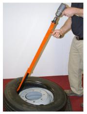
Begin to extend the push foot with an impact wrench in a counter clockwise motion. As the pushing foot begins to meet the rim, ensure that the plastic protective angle properly engages the rim edge and allow the natural motion of the tool to rock backwards.
