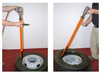
Continue to retract the pulling foot with the impact wrench while bringing the tool towards the wheel center in a pivoting motion until the 1st bead is removed. NOTE: Do not force or excessively pry with the tool. Allow the natural motion of the pulling foot to remove the tire.
