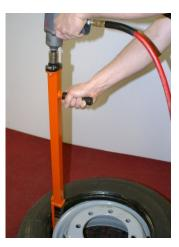
When the first bead is removed, turn the impact tool in a clockwise motion too reset the pushing arm.
