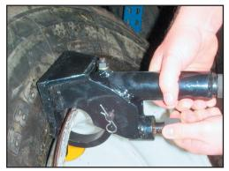
3. Tighten rim clamp jaw until "snug" with hand wrench. Make sure bead breaker teeth and foot are against bead.
