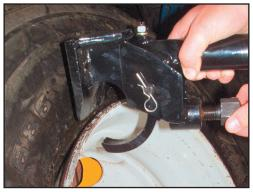
2. Place bead breaker onto the rim with teeth and breaker foot between rim & tire bead.
