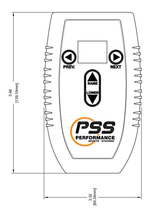
UNIT IS DESIGNED TO OPERATE UP TO 99 REMOTE RECEIVERS MODEL 1199.
