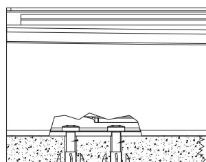
Schraube M6 (1/4" thru-bolt and tee nuts)
