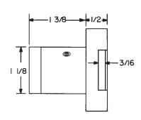
Use of spacers and strikes depends on application and material thickness.
