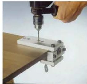
Drill the adjustment hole.
