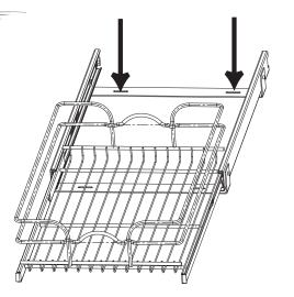
**Step 2.** Slide drawer out half way to allow for installation of rear screws into cabinet floor.
