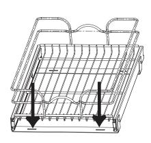
**Step 3**. Install front slides to cabinet floor with provided screws
