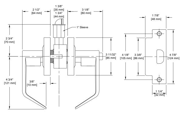
Door Prep: Cross Bore 2 1/8+, Edge Bore 1+, Latch Face 1 1/8+x 2 1/4+
