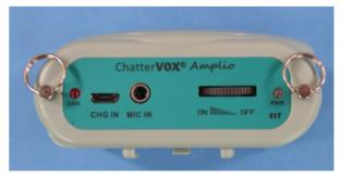
CHG: RED LED turns on when charging. LED turns off when charged CHG IN: micro-USB 5-6VDC
