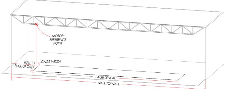
Figure 5: Rendering of Motor Reference Point Location
