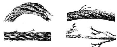
Figure 2: Worn and Damaged Wire Ropes - Replacements Required
