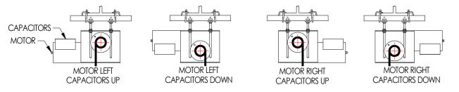
Figure 19: Rendering of Proper Cable Wrapping in Relation to Winch Rotation
