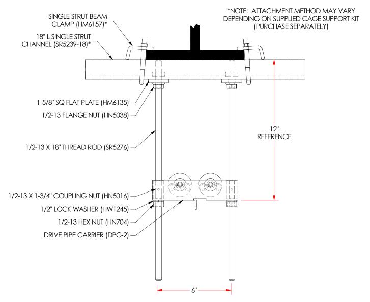
Figure 11: Rendering of Drive Pipe Carrier Assembly, DPC-A (Section B-B)
