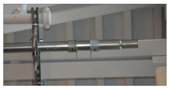
Figure 13: First Drive Pipe Segment and Cable Guide Installation
