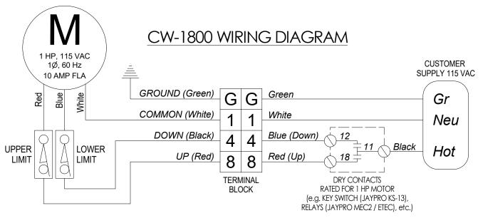
Figure 27: Winch (CW-1800) Wiring Diagram for Key Switch (KS-13) Operation
