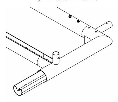
Figure 2: Assemble Both Corner Piece
