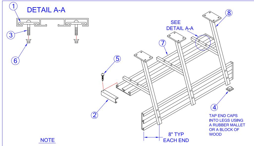
DUE TO THE WIDE VARIATIONS IN FLOOR CONSTRUCTION AND MATERIALS, LEG ANCHORS AND ASSOCIATED HARD-WARE ARE NOT PROVIDED. IT IS THE INSTALLERS RESPONSIBILITY TO DETERMINE THE SUITABILITY OF THE FASTENERS.
