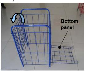
3. Place the carrier upside down. Turn the bottom panel to the bottom of carrier. Push the bottom panel all the way to make sure the wire grid tab fits over and onto the bottom grid for side panel.
