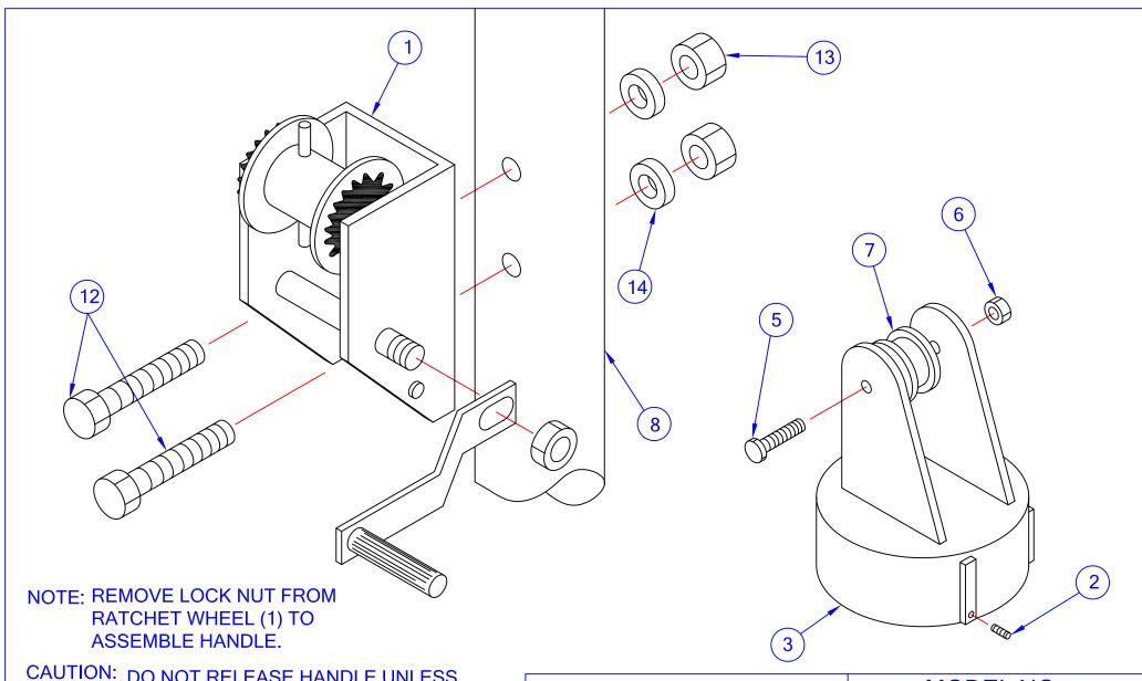
CAUTION: DO NOT RELEASE HANDLE UNLESS RATCHET PAWL IS PROPERLY ENGAGED. DO NOT DISENGAGE RATCHET PAWL UNLESS TENSION IS APPLIED TO HANDLE. FAILURE TO OBSERVE THESE CAUTIONS WILL CAUSE HANDLE TO SPIN OUT OF CONTROL AND COULD CAUSE PERSONAL INJURY.
