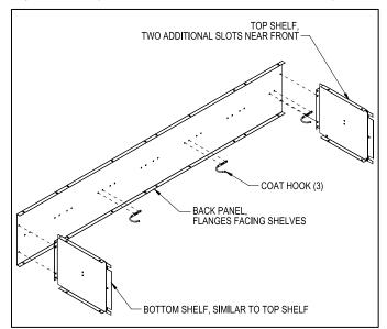
**Step 2:** Turn the back panel onto its back with the shelves pointing upward. Attach the first side panel, the left rear leg, and two compartment dividers to the assembly from Step 1. Attach three additional coat hooks to the first side panel.
