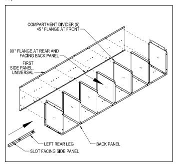
**Step 3:** Attach the second side panel and the right rear leg to the assembly from Step 2. The locker chassis is now complete.
