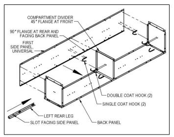
**Step 3:** Attach the second side panel and the right rear leg to the assembly of Step 2. Attach an additional two single coat hooks to the second side panel. The locker chassis is now complete.
