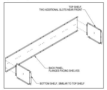
Step 2: Turn the back panel onto its back with the shelves pointing upward. Attach the first side panel, the left rear leg, and five compartment dividers to the assembly from Step 1.
