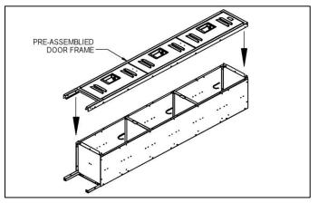
**Step 5:** Tighten all fasteners checking for squareness of the locker while tightening. Attach optional sloping hood, end bases or front bases (see pages 4 and 5).
