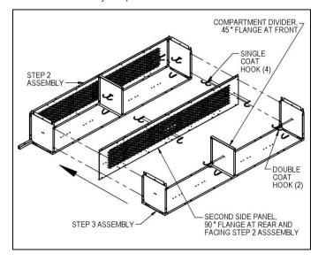
**Step 5:** Attach the third top shelf, the third bottom shelf, and an additional two coat hooks to the third back panel as in steps 1 and 3.
