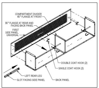
**Step 3:** Attach the second top shelf, the second bottom shelf, and an additional two single coat hooks to the second back panel as in step 1.
