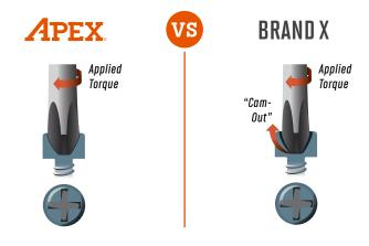
Precision fit of APEX tools eliminates "camout" and premature bit failure.
