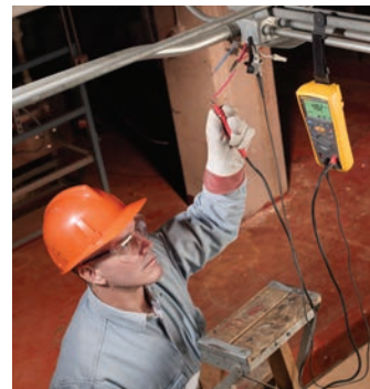
Magnetic Meter Hanger frees up both hands to focus on making measurements safely.
