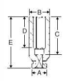
A special 1-3/4" extra deep impact socket for applications where a deep impact socket will not reach the fastener.
