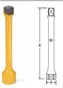
Provides the ability to torque inner and outer cap nuts and flange nuts on heavy duty trucks using an impact wrench and our standard or heavy duty impact sockets.
