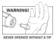
**Select Tip:** Insert tip into electrode bore making sure of positive contact. **Select Puller type:** Chose 2.2 or 2.6 Uni-stud, straight or twisted Uni-tab. Be certain to fully insert pin or tab into tip. DO NOT USE PANEL TO PUSH!!
