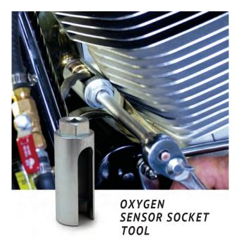
This tool is used to remove or install the oxygen sensor on all closed loop fuel injected H-D $^\circ$  models. Socket has a 3/8" drive receiver or can be used with a 7/8" wrench. Socket will withstand up to 125 ft/lbs of torque.
