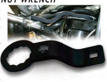
us with a great flat rate time saver stem nut tool for use on Touring Model Harleys. Normally to get access to the top stem nut you would need to remove the radio package. With this tool you are able to loosen, tighten and torque to spec. the 1-1/2" stem nut without radio removal and ultimately saving you 45 minutes for an experienced mechanic! For more details see No.977-IS instructions.
