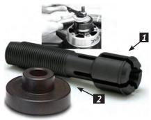
This tool is used to remove and install the new front 25mm H-D° bearing, including ABS or non ABS wheel bearings on most of the 2007 to present with 25mm bearing models. Note: This tool must be used
