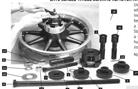
Use to remove and install "new style" sealed wheel bearings without damaging the wheel. Includes new remover and installer for 25mm bearing, with or without ABS. Also included is a 30 pack of "surface Temperature Indicating Strips." These are used to assist in removing a stubborn bearing when applying heat to a hub surface. For more details see No.1042-IS instructions.
