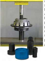
and installs the clutch shell ball bearing (H-D° No.37906-90) without any damage to the new bearing. This is done by pushing on the outer perimeter of bearing. For more details see No.971-IS instructions. No.**971** - Use on all
