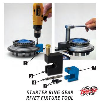
This tool is designed to remove the starter ring gear rivets from Big Twin clutch shells to install JIMS<sup>®</sup> No. 639 and 640 or equivalent performance starter ring gears. *For more details see No.965-IS instructions*.
