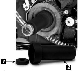
This tool will easily remove and install the right hand threaded nut that holds the trans pulley on. The inner collar No. 1 is designed to be threaded onto the left-hand thread of the main shaft. With the inner collar in place, this will stop the tool from slipping when torquing the nut. See H-D® Service Manual for torque specs. Apply lube to threads of tool.
