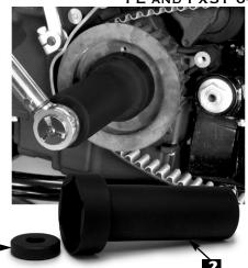
This tool will easily remove and install the right hand threaded nut that holds the trans pulley on. The inner collar No. 1 is designed to be threaded onto the left-hand thread of the main shaft. With the inner collar in place, this will stop the tool from slipping when torquing the nut. See H-D® Service Manual for torque specs. Apply lube to threads of tool.
