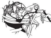
CHECKING VACUUM ADVANCE CHAMBER
