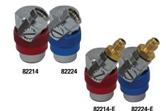
This unique patented design easily snaps on and off the A/C systems service ports under any pressure. The E-Z Snap™ automatically adjusts to various service port dimensions allowing fast and immediate access into the A/C system. The swivel feature enables the user to easily access all service ports, even in the tightest quarters. Meets SAE, UL, and EPA requirements for containment of refrigerant. **PATENT# 5,244,010**
