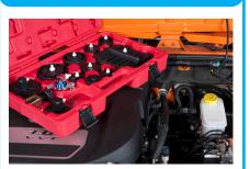
The Master Cylinder Cover Kit contains 12 universal and manufacturer-specific adapters designed to fit 90% of the current master cylinder reservoirs found in vehicles. This kit is required for most brake flush applications and mandatory for the pedal assist flush.
