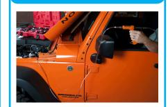
In our quest to developing the quickest brake flush technique, we developed the XL flush hose to allow the Phoenix bleeder to pressurize the master cylinder while depressing the brake pedal for a pedal assist flush. We invented this technique right here at Phoenix Systems.
