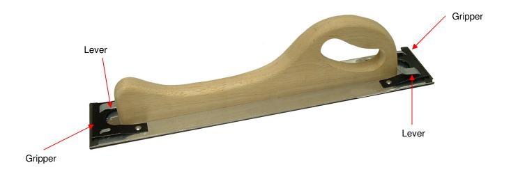
Have a 23/4" x 171/2" standard cut abrasive sheet. Raise one lever so it is at a right angle to the base. Insert the sheet of sandpaper under the gripper. Return the lever to the original position. Raise the second lever so it is at a right angle to the base. Wrap the sandpaper around the bottom of the base under the second gripper. Return the second lever to the original position.
