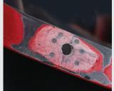
Sand with a P80 – P180 grit disc to desired shape & drill as needed.
