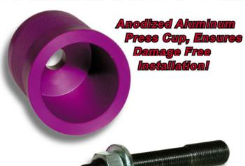
This Special Kit was designed for the proper installation of **Pulley Crank Shaft** oil seals. The step bolt screws into the crank shaft end. The press nut w/ washer allows for an even pressing force, seating the oil seal into the engine case every time.
