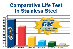
Average Number of Holes Before Failure (in 16 gauge stainless steel plate)
