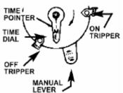
TIMES: Hold TRIPPERS against edge of CLOCK-DIAL, pointing to time (AM or PM) when **ON** and **OFF** operations are desired. Tighten tripper screws firmly.
