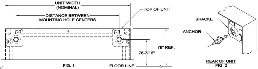
TO MOUNT A 96" LONG UNIT, USE THE "L"-HANGERS (PROVIDED) IN ADDITION TO WALL ANCHORS (NOT PROVIDED) AND FOLLOW THE MOUNTING INSTRUCTIONS ENCLOSED WITH IN THE "L"-HANGERS.
