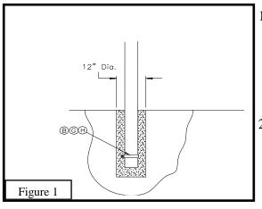
1. Select the location for the concrete base footing. Dig a 12" diameter hole that is a minimum of 48"deep. In areas where the normal frost line is below 48" it is advisable to dig to the normal frost line. (Consult a local concrete contractor if there is any question.)
