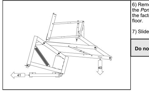
6) Remove the *Shipping Pallet* by tilting the *Portable Base Assembly* (A) back until the factory installed wheels contact the floor.
