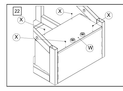
22) Install *Weight Box Lid* (W) with four #12-14 x 3/4" Hex Washer Head Sheet Metal Screws (X).
