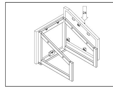
24) Install *Front and Side Pads* (Z) by hooking *Padding Brackets* (AA) onto *Portable Base Assembly* (A). Tighten the set screws on the *Padding Brackets* (AA).
