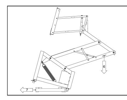
6) Remove the *Shipping Pallet* by tilting the *Portable Base Assembly* (A) back until the factory installed wheels contact the floor.
