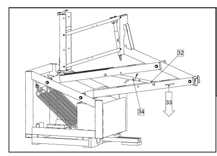
32) Remove *Hitch Pin* from *Up Position Hole*.
