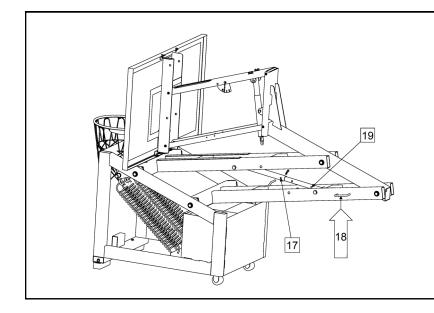
17) Remove *Hitch Pin* from *Down Position Hole.*
