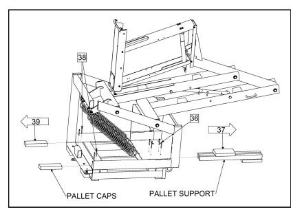
36) Remove four Hex Drive Wood Screws from inside *Weight Box.*
