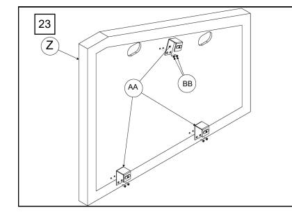
23) Install 3 *Padding Brackets* (AA) onto *Front and Side Pads* (Z) using two *1/4" x 3/4" Phillips Drive Flat Head Screws* (BB) in each bracket.
