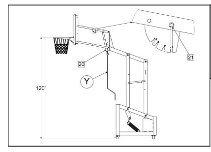
20) Using *Crank Handle* (Y), raise *Goal Height Adjuster* until the *Goal* (O) is 10ft from the playing surface.
