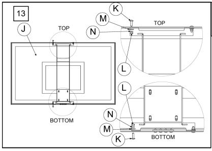
13) Install *Backboard* (J) using the supplied hardware (K-L) at each of the four locations.
