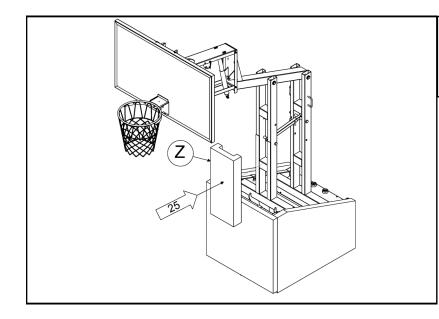
25) Install *Upright Pad* (Z) by pressing onto the existing hook and loop strips on the front of the *Uprights.*
