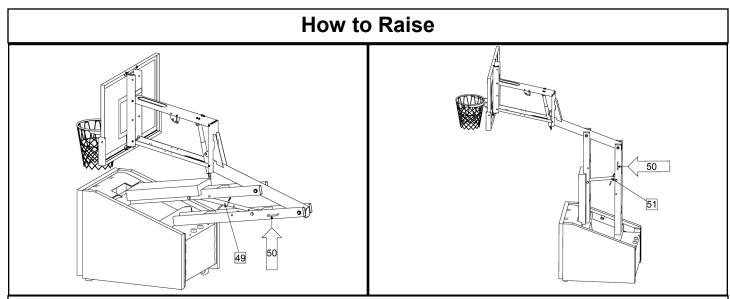
49) Remove Hitch Pin from Down Position Hole.
