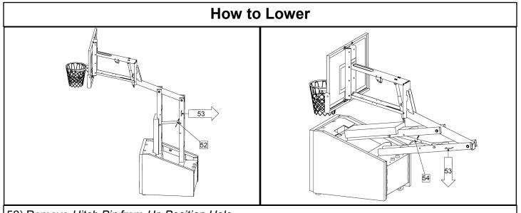
52) Remove Hitch Pin from Up Position Hole.
