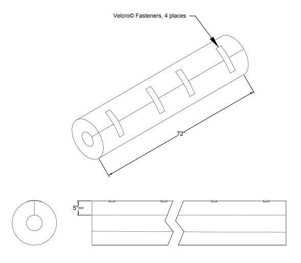
Padding shall meet all NCAA and National High School Federation rules. Foam shall be a minimum of 5" thick and be covered with sewn vinyl covering in 16 school colors. Height shall be 72" minimum and be designed to attach by means of Velcro fasteners to all goalposts up to 5 9/16" diameter or 4" square. Installation to be completed in accordance with manufacturer's instructions. Shipping weight shall be 18# each.
