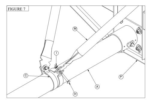
12a. If you are installing PR75 or PR75XL system with a BA475SS Backboard, use 3/8" x 1" Hex Bolts (E), 3/8" Flat Washers (F), and 3/8" Lock Washers (G) to attach the other end of the Backboard Braces (M) to the threaded holes in the rear of the Backboard (P). See Figure 8.
