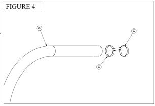
9. Place the assembly from 7a or 7b above on to the end of the pole. It is easiest to place the assembly onto the end of the pole upside down and then rotate 180° before installing and tensioning the 1/2" Square Head Set Screws (N). Confirm that the Rim (Q) and Backboard (P) are level. Tighten the 1/2" Square Head Set Screws (N) against the Gooseneck Pole (A), then tighten the 1/2" Jam Nuts (O) to lock the 1/2" Square Head Set Screws (N) See Figure 5 and Figure 6.
