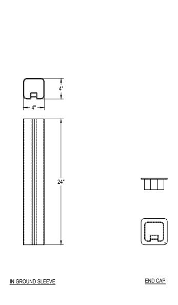
Sleeves shall be constructed of 6063-T6 extruded aluminum and require bury in an 8" x 30" minimum footing. Actual sleeve depth shall be 24" and be designed to allow removal of 4" square uprights on Bison in-ground soccer goals. Sleeve shall have a removable steel top cap. Installation to be completed in accordance to manufacturer's instructions. Do not scale drawings. Weight approximately 5#/each.
