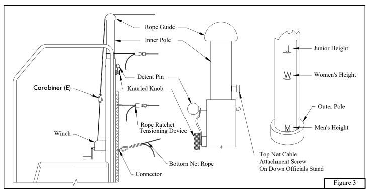
10. Move one of the factory installed connectors 2-3" below the bottom of *Net* (C) on both *VB81*Standards (A). Attach rope ratchet device on the bottom rope to the winch end connector, attach the other end of the bottom rope to the non-winch end connector using one of the *Carabiners* (E) provided in the hardware kit.
