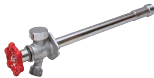
Anti-Siphon Frost Free Sillcock Chrome-Plated Brass 3/4" Male & 1/2" Female Multi-turn | Anti-Siphon
