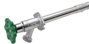
No Lead Frost Free Sillcock Chrome-Plated Brass 1/2" Male & 1/2" Solder Multi-turn
