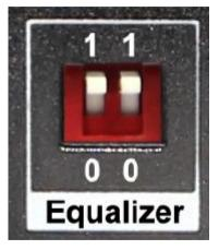
If you see flickering or blinking image on the display, adjust the EQ switch to improve the cable skew. MAX stands for the strongest HDMI signal level for the longest possible transmission length while MIN stands for the weakest HDMI signal level for short transmission length. Adjust the signal level from MIN to MAX until desired video quality is displayed.
